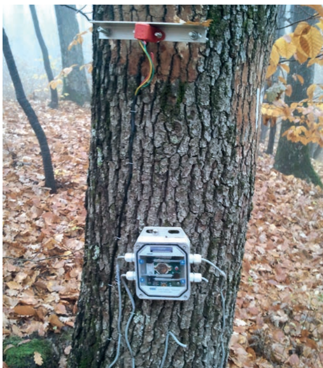
Figure 3-4: Point dendrometer mounted on an oak tree.
