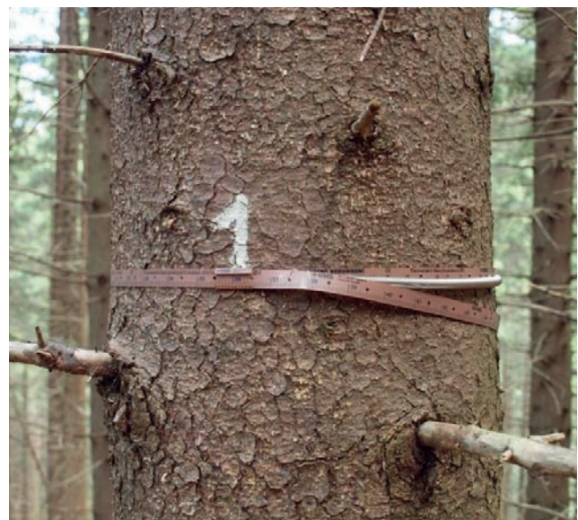
Figure 3-3: Permanent girth band mounted on a Norway spruce tree.
