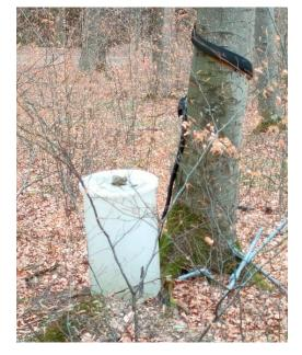
Figure 6-1: Throughfall samplers (left) and stemflow sampler (right) on Level II plot 'Klausen-Leopoldsdorf' in European beech (*Fagus sylvatica*) stand located west of Vienna, Austria. Images: Arne Verstraeten
